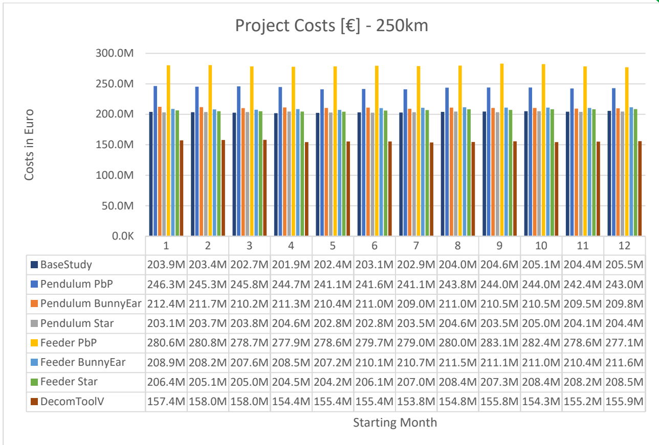
Figure 8: average costs of different configurations at a distance of 250 km over a period of one year – complete supply chain (1-12 equals the months from January to December)
