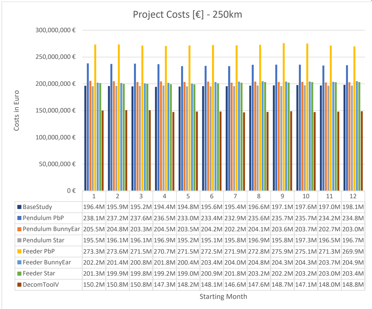
Figure 20: average costs of different configurations at a distance of 250 km over a period of one year – offshore (1-12 equals the months from January to December)
