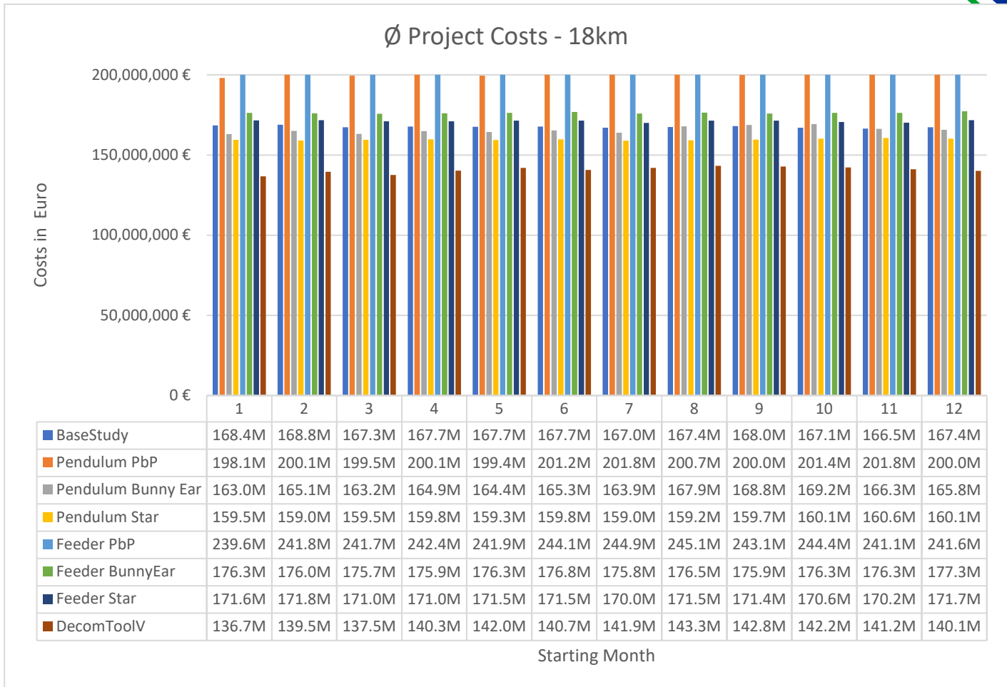
Figure 2: average costs of different configurations at a distance of 18 km over a period of one year – complete supply chain (1-12 equals the months from January to December)
